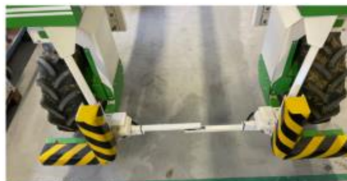
On the TED straddler, a detection system has been patented. When a human stands on the vine row, it triggers a safety stop.
